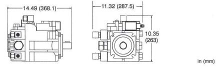
**Note:** This outline drawing is provided for general reference only and is not intended for design or installation. For more information see Operation and Installation manuals or obtain drawing 500-3763 and wiring diagram from your distributor/dealer.
